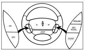
The speed control switches on the steering wheel
